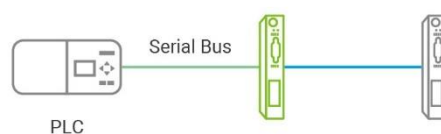
Figure 5-2 CR5201B/SE5201B is set as a TCP Server Link Mode
