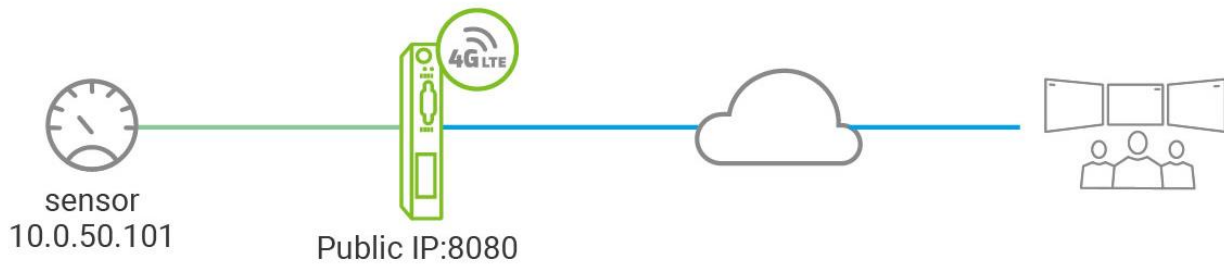
Figure 4-23 Example of Port Forwarding through SE5201B Low-Power Gateway
