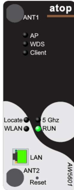
Figure 6.6.4. Locate Turn-off State on Panel
